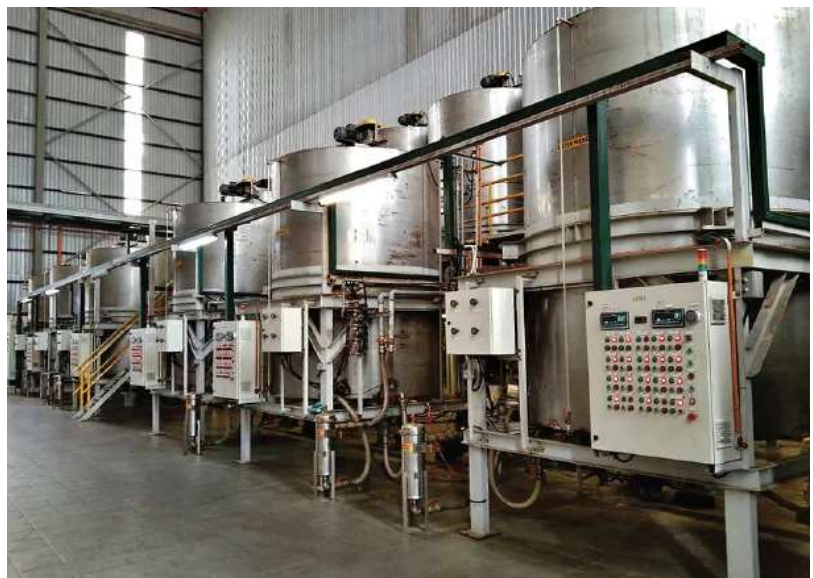
Latex-mixing equipment used in glove manufacturing
